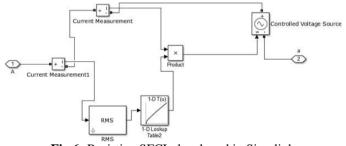
Fig 6: Resistive SFCL developed in Simulink
