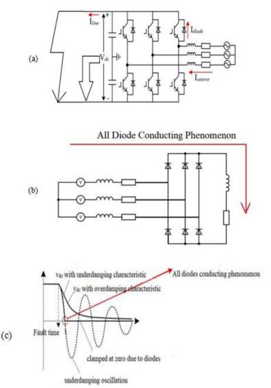
Fig 4(a,b,c): Equivalent circuit of the dc pole-to-pole fault and the transient characteristics of the dcvoltage.
