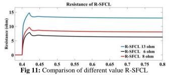
From fig. 11. It is clear that the at fault time t=.4sec the resistance of R-SFCL is build up 13,6 and 8 for suppressing the fault current. The above simulation analysis can be used as the basis for parameter selection of the R-SFCL in practical application.
