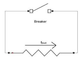
Resistance Fig 3b: During the fault operation process
